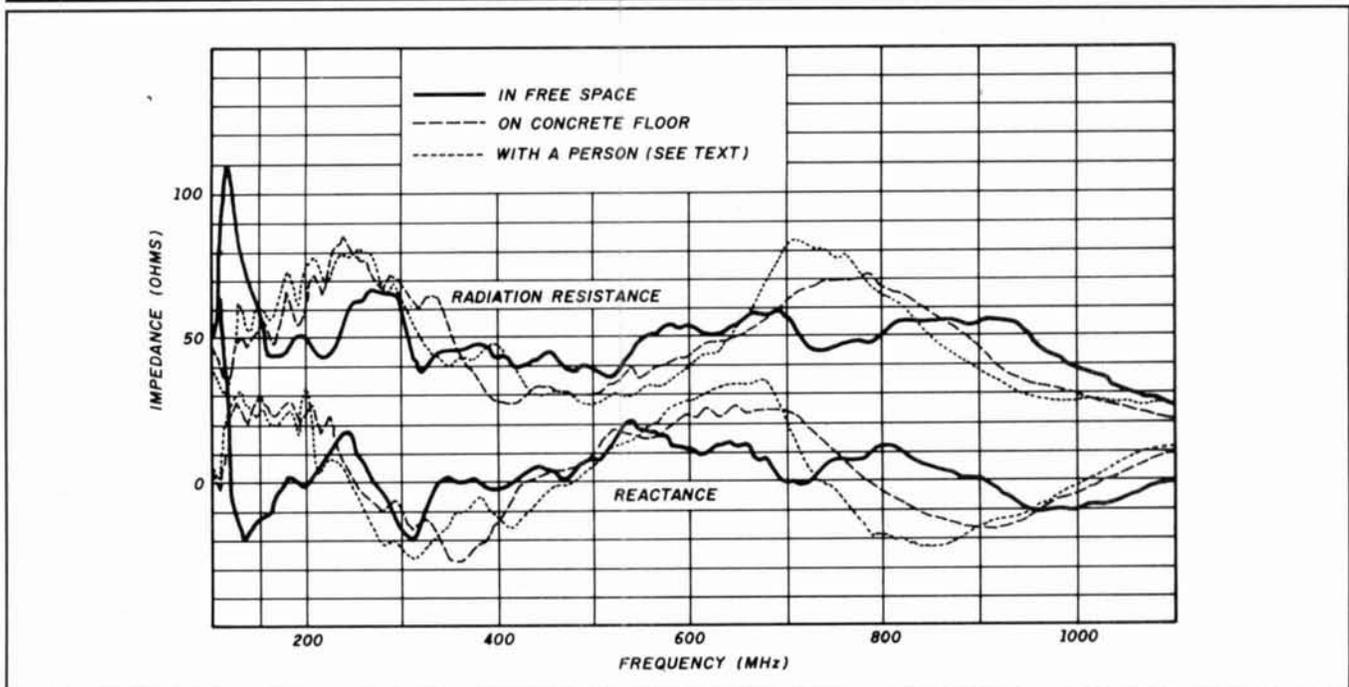
Impedance versus frequency of a symmetrical Heart antenna. (Antenna is made from sheet aluminum 1.5 mm thick.)
