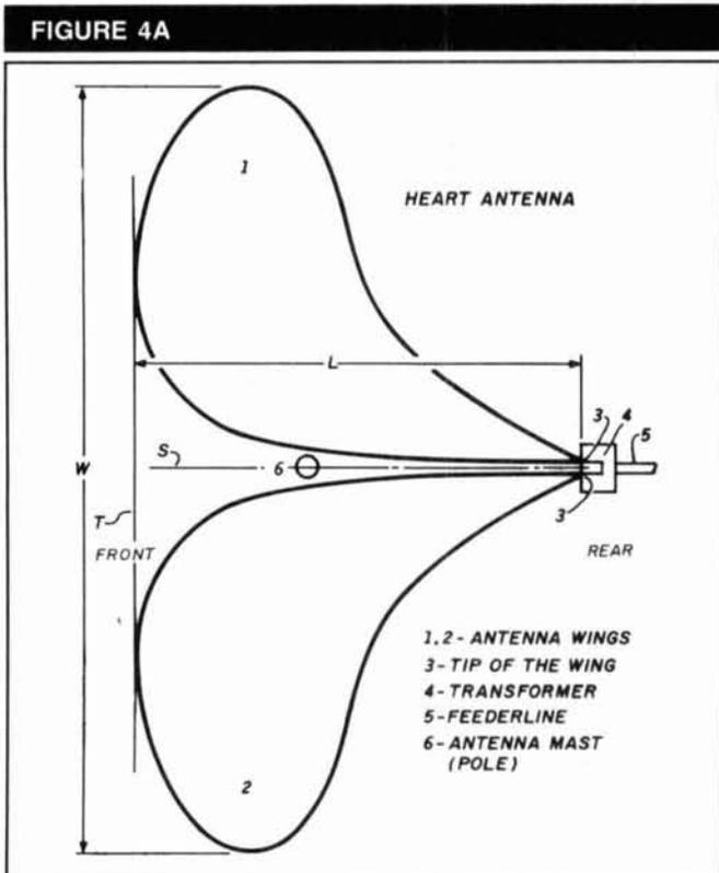
Symmetrical Heart antenna (showing both wing profiles).
